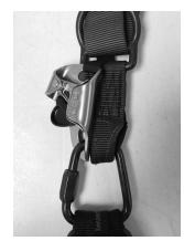
Insert rope into chest ascender for rope ascending techniques. Tighten chest strap for ascending mode.
